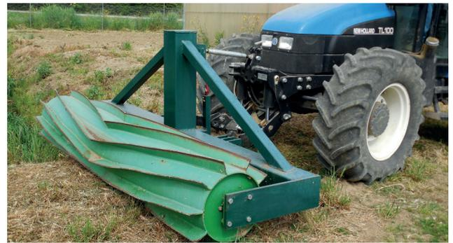
**Figure 1** - The Rodale Institute design-based roller crimper front-mounted at the tractor.
