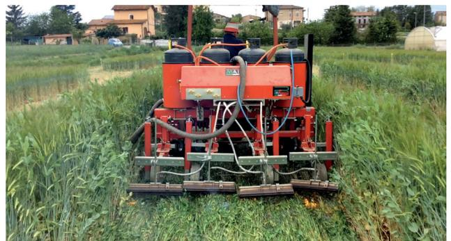
**Figure 2** - A flaming machine terminating cover crops after the roller crimper has been used.
